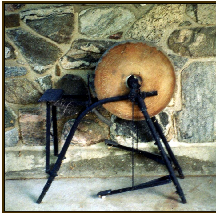
Allie used this foot pedaled grinding stone to sharpen the hay mower knives
